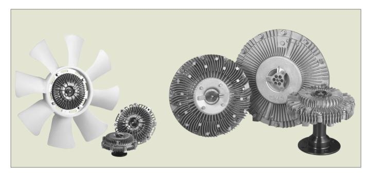
Fan clutches reduce the drain of engine horsepower and improve the efficiency of a vehicle's cooling system. Fan clutches are fluid coupling devices which provide air flow through the radiator by using the water pump shaft to power a rigid fan blade. Fan clutches are available in thermal and non-thermal designs.
